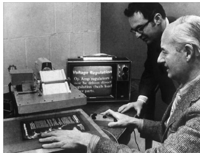
Figure 3. The closed-circuit-television (CCTV) reader for the visually impaired, a bachelor thesis product by two MIT seniors. Unlike current commercial versions, the control panel I am operating with my right hand moves the copy under the TV camera.
